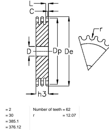
C = 2 D = 30 De = 385.1Dp = 376.12For chain size =  $3/4 \times 7/16$ For chain type = 12 B-3h3 = 49.8L = 10.8
